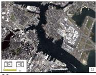
Now we have zoomed to the limit of resolution of the Landsat image. This image is pixelated. We can't see anything smaller than 30 meters (100 ft) on a side. We'll look at another satellite image with higher resolution - IKONOS. It has 4 meter resolution. If we looked at 1 Landsat pixel, how many pixels would that become on an IKONOS image?
