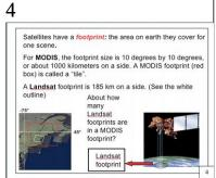
The footprint of Landsat is the white outline. Ask your students to estimate how many white boxes can fit in the blue box, the outline for one MODIS scene (tile). One Landsat scene is about 200 km "square" and so 5 could fit along the MODIS tile width dimension of 1000 km, and 5 along its height. So that would be about 5x5 = 25 Landsat scenes in one MODIS tile. Have your students try this on graph paper or with to scale cut-outs.
